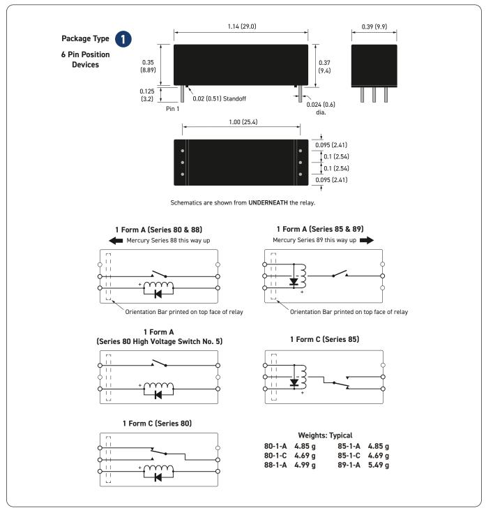
**Important:** Where the optional internal diode is fitted or for all Form B types, the correct coil polarity must be observed as shown by the + symbol on the schematics.
