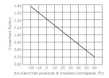
To use this chart: Read up from the ambient temperature to the curve, and across to find a correction factor. Multiply the breaker rating by the correction factor to determine the compensated rating. Calculate the overloads in terms of the compensated rating to use the published trip curve. Do not use these devices outside their specified
