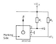
For optimum protection against destruction,  $R_{\rm s}$  is required to be as high as possible. Dimensioning:
