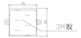
3. Srew installation. Please use ⊄3 screw to fix the mounting hole to corresponding place as below
