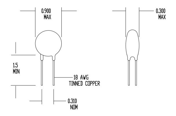
RESISTANCE AT 25 DEG C = 2.5 DHMS +/- 15% MAX CONTINUOUS CURRENT (Imax) = 10 AMPS RESISTANCE AT Imax = 0.04 DHMS NOMINAL MAX VOLTAGE RATING = 265 VAC (RMS) MAX SURGE RATING = 87 JOULES
