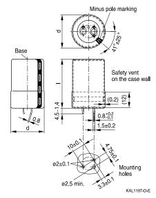
Snap-in capacitors are also available with 3 terminals (length (4.5 -1.4) mm). PET insulation cap is positioned under the insulation sleeve.
