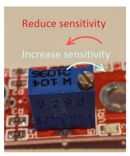
This sensor doesn't show absolute values (like exact temperature in °C or magneticfield strenght in mT). It is a relative measurement: you define an extreme value to a given normal environment situation and a signal will be send if the measurement exceeds the extreme value.
