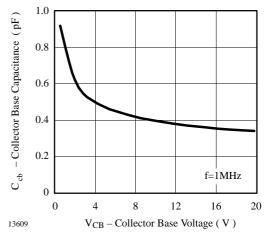
Figure 3. Collector Base Capacitance vs. Collector Base Voltage
