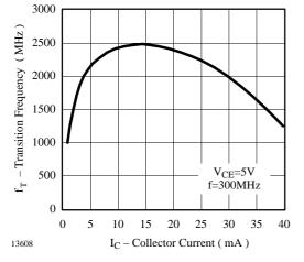
Figure 2. Transition Frequency vs. Collector Current
