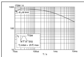
Fig.2. Maximum permissible non-repetitive peak on-state current  $I_{TSM}$ , versus pulse width  $t_p$ , for sinusoidal currents,  $t_p \le 10$ ms.
