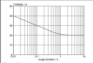
Fig.5. Maximum permissible repetitive rms on-state current  $I_{T(RMS)}$ , versus surge duration, for sinusoidal currents, f = 50 Hz;  $T_{mb} \le 103$  °C.
