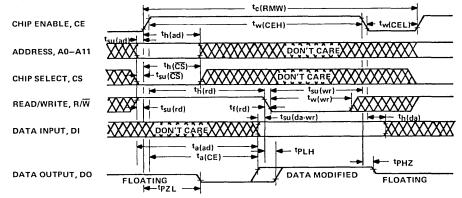
NOTE: For the chip enable input, high and low timing points are 90% and 10% of VIH(CE). Other input timing points are 0.6 V (low) and 2.2 V (high). Output timing points are 0.4 V (low) and 2.4 V (high).
