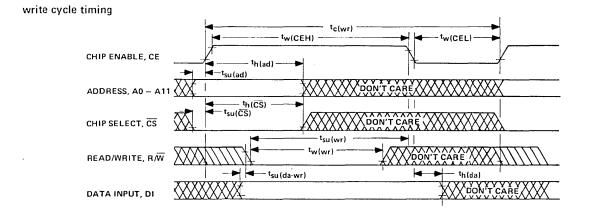
NOTE: For the chip-enable input, high and low timing points are 90% and 10% of V<sub>1H(CE)</sub>. Other input timing points are 0.6 V (low) and 2.2 V (high). Output timing points are 0.4 V (low) and 2.4 V (high). During the time from the rise of CE to the fall of R/W, R/W is permitted to change from high to low only.
