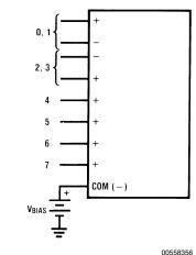
FIGURE 1. Analog Input Multiplexer Options for the ADC0838
