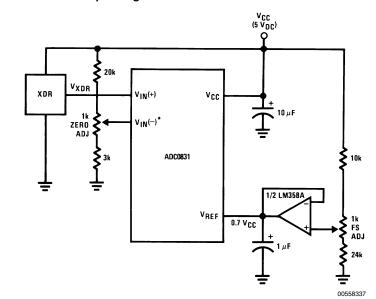
$^{*}V_{IN}(-)$  = 0.15 V\_CC 15% of V\_CC  $\leq$  V\_XDR  $\leq$  85% of V\_CC
