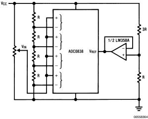
Controller performs a routine to determine which input polarity (9-bit example) or which channel pair (10-bit example) provides a non-zero output code. This information provides the extra bits.
