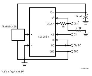
FIGURE 7. Remote Sensing -Clock and Power on 1 Wire
