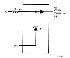
FIGURE 3. An On-Chip Shunt Regulator Diode
