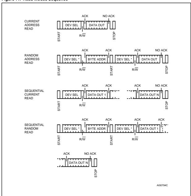
Note: \* The 7 Most Significant bits of DEV SEL bytes of a Random Read (1st byte and 3rd byte) must be identical.
