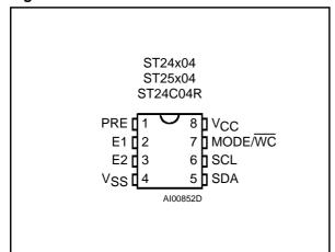
Figure 2B. SO Pin Connections
