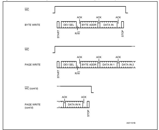
Figure 10. Write Modes Sequence with Write Control = 1 (ST24/25W04)
