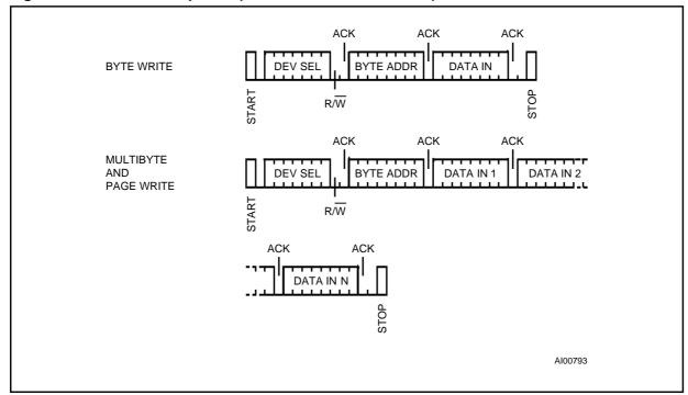
Figure 9. Write Modes Sequence (ST24/25C04 and ST24C04R)
