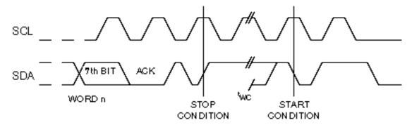
Note: The write cycle time t<sub>wc</sub> is the time from a valid stop condition of a write sequence to the end of the internal clear / write cycle.
