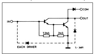
For ULN2803A (each driver for 5 V, TTL/CMOS)
