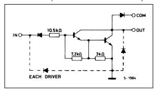
For ULN2804A (each driver for 6-15 V CMOS/PMOS
