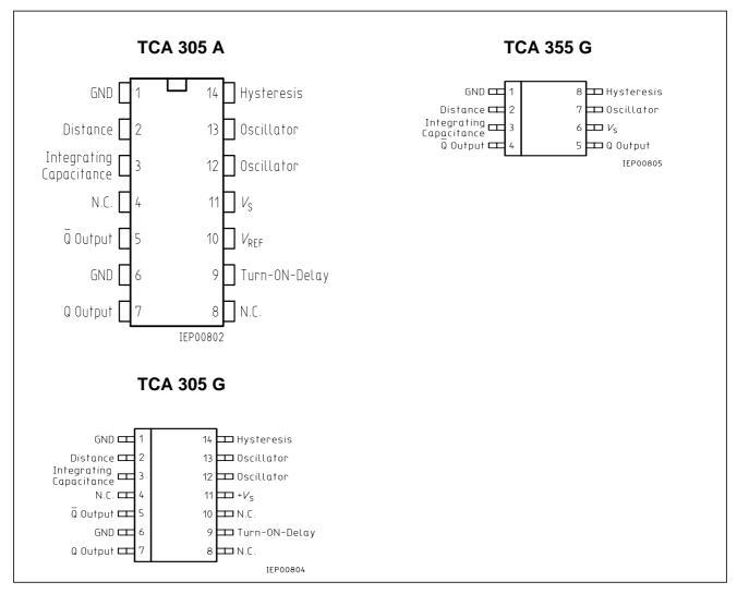
Pin Configurations (top view)
