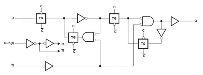
Figure 8-2. Logic Diagram, each flip-flop (potitive logic)
