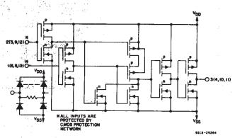
Fig. 1 - Schematic diagram for CD4081B (1 of 4 identical gates).
