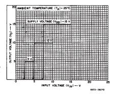
Fig. 3 - Typical voltage transfer characteristics.
