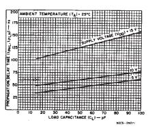
Fig. 4 — Typical propagation delay time as a function of load capacitance.
