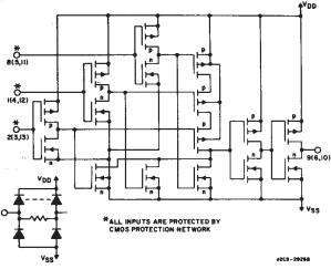
Fig. 11 — Schematic diagram for CD4073B (1 of 3 identical gates).
