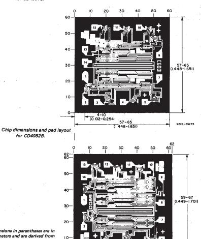
Dimensions in parentheses are in millimeters and are derived from the basic inch dimensions as indicated. Grid graduations are in mils (10<sup>-3</sup> inch).
