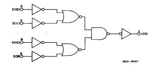
Fig. 9 - Logic diagram for CD4082B (1 of 2 identical gates).
