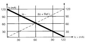
For single-ended operation with capacitive loads use a reverse-biased diode (IN914, IN4148, IN4001, etc.) across each output to output common, i.e., any combination of +lo and -lo which does not exceed a total of 120mA. Output noise and load regulation will degrade linearly to 4mV rms, and 1.0% with single-ended operation.
